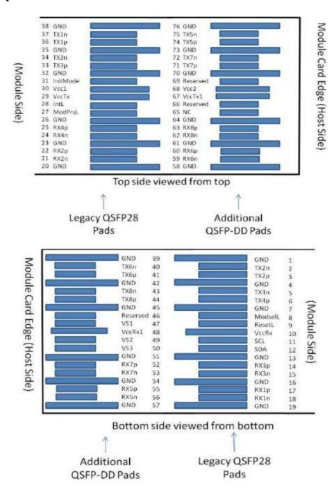
**QSFP-DD** compliant 76 pin connector
